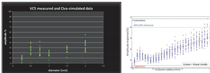
Sensitivity calibration was performed by a flat bottom hole of diameter 0.4mm located in an N18 block (powder metallurgy) located at the same depth as the respective spherical defects.
