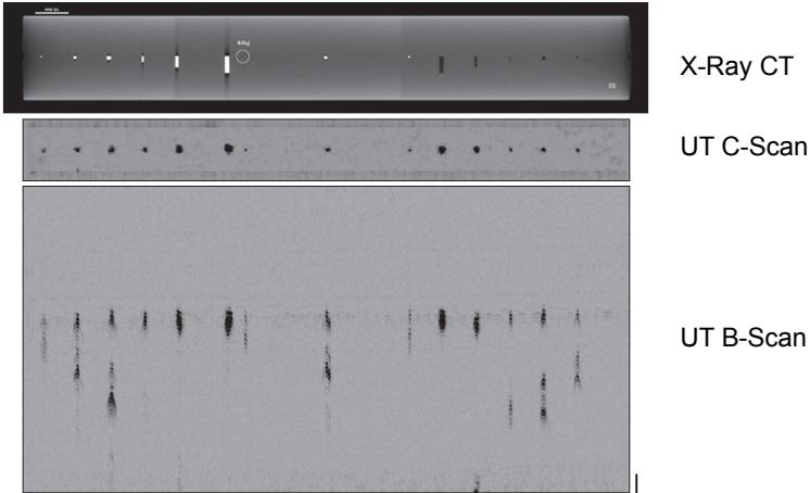
Reference measurements of artificial flaws by X-Ray CT and ultrasonic B- and C-Scans at 20 MHz.
