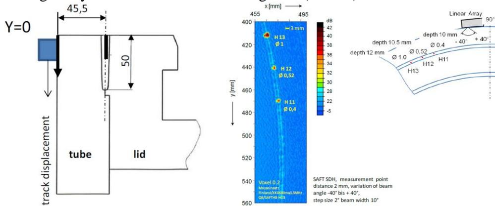
**Figure 6:** Evaluation and sizing of electron beam weld defects by PC-SAFT
