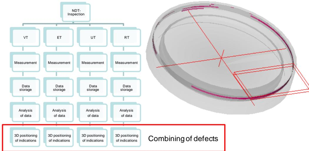
**Figure 10:** Combining of indications with four NDT methods
