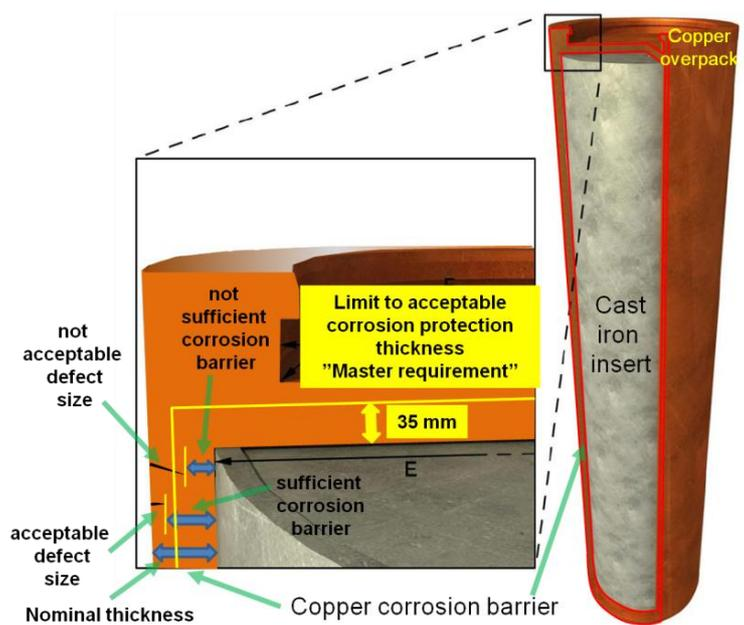
**Figure 13:** Master requirement of the disposal canister for acceptance rejection process.
