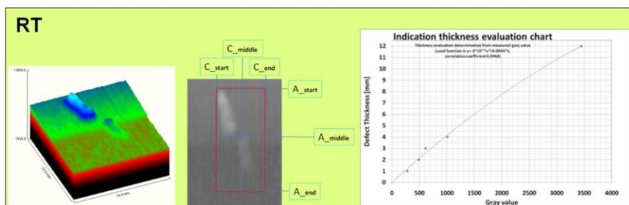
**Figure 7:** Evaluation and sizing of radiographic indication
