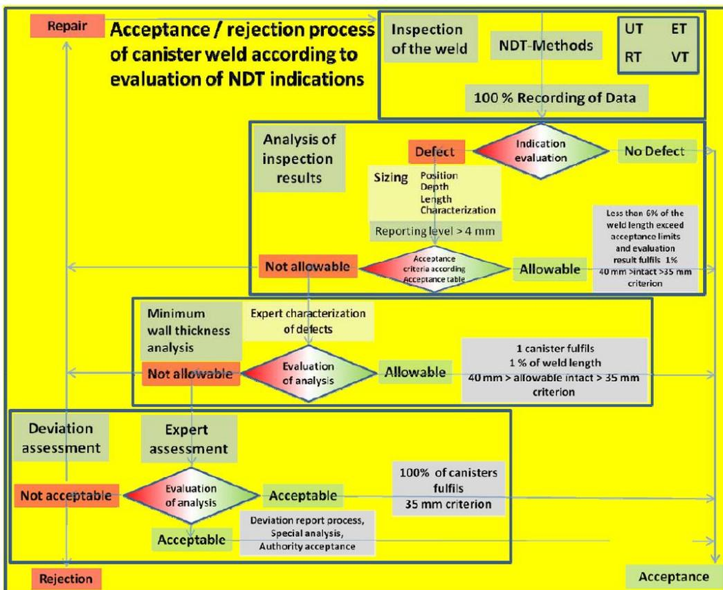
**Figure 14:** Acceptance and rejection process of copper components according to the evaluation of NDT indications.
