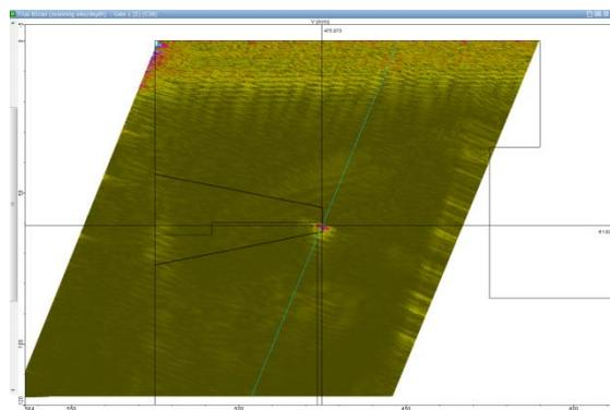
**Figure 3:** Raw data evaluation of phased array ultrasonic data
