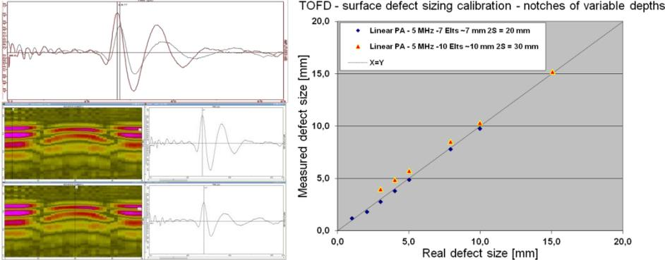
Figure 5: Evaluation and sizing with TOFD calibration
