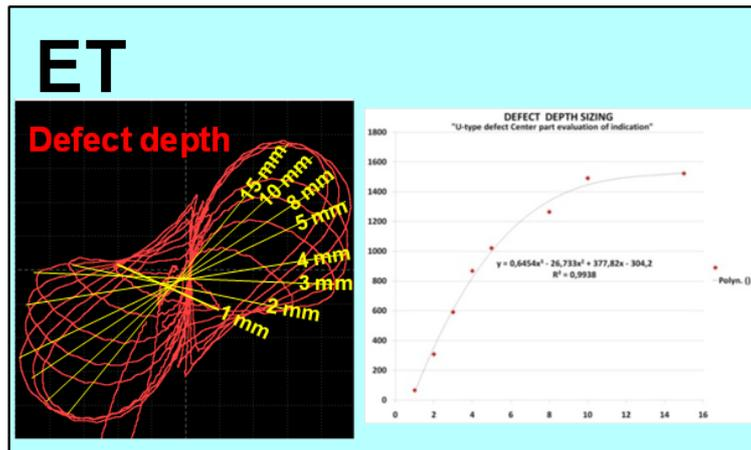
Figure 8: Evaluation and sizing of eddy current Indication
