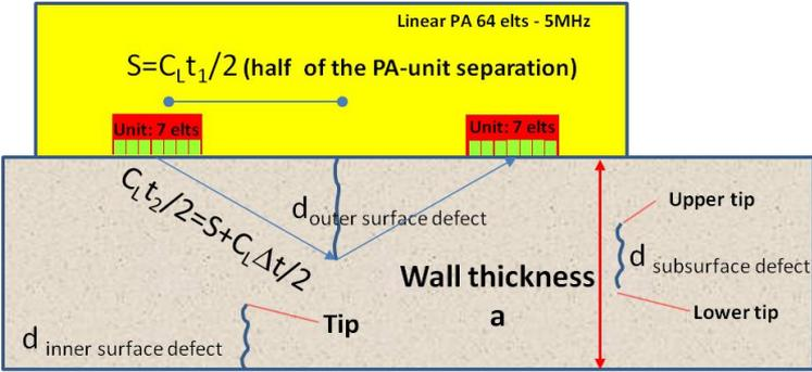
Figure 4: TOFD measurement set up for a phased array probe
