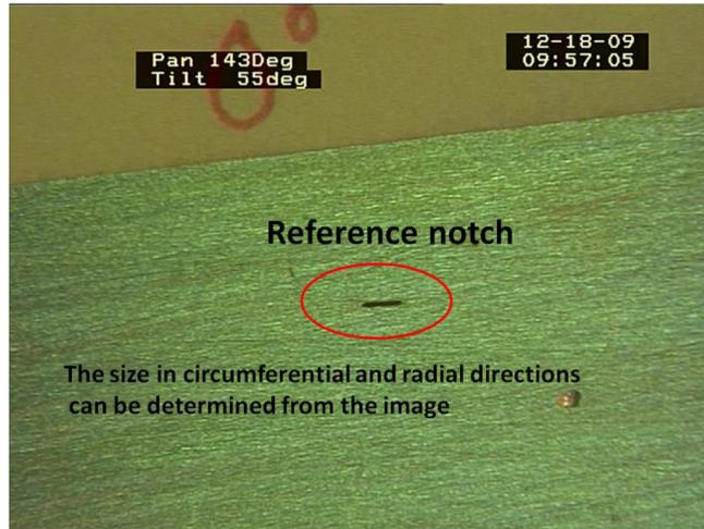
**Figure 9:** Visibility of 0.1 x 1.5 mm (w x l) notch with 7.5 x magnifications (0.5 %s)
