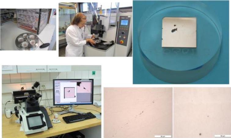
**Figure 1:** Metallographic study of detected defects
