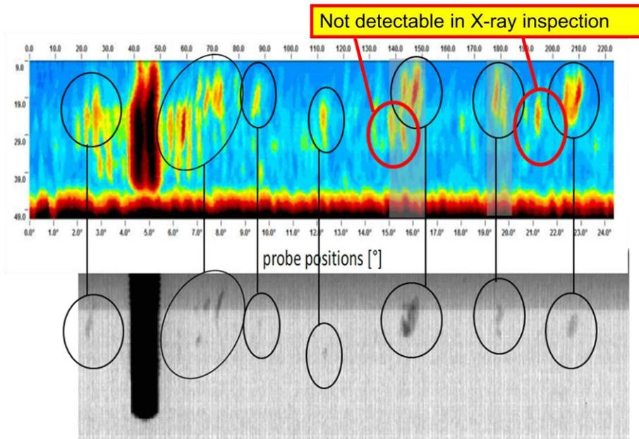
**Figure 12:** images of real defects by applying PA-SAFT (C-scan in upper part of the image) and X-ray image (lower part of the image)
