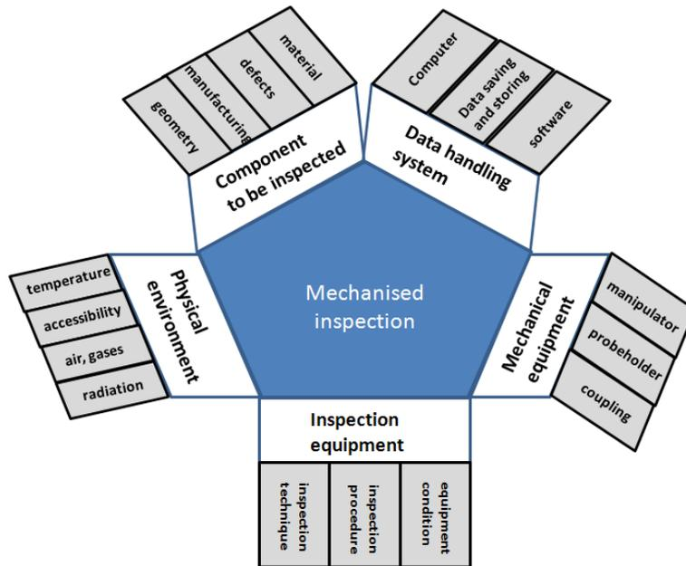
**Figure 2:** Technical parameters affecting the reliability of mechanized inspections
