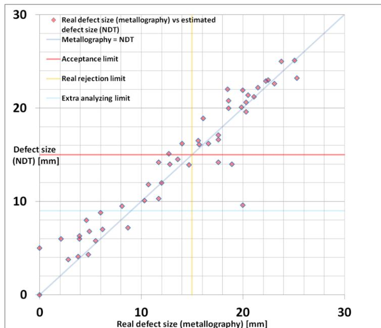
**Figure 11:** Metallographic size compared to defect size received in NDT evaluation
