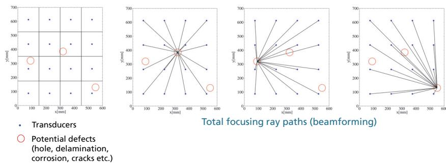
SHM sensor network in total focusing mode can be considered as a special case of an ultrasonic scanning device!
