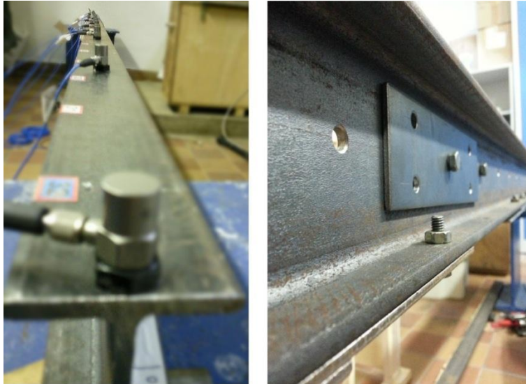
Pic. 5. Physical model showing the deploying of the sensors and damage model
