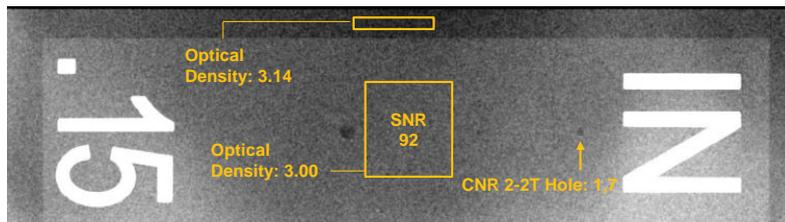
2-2T Hole  $\triangleq$  Defect with  $\varnothing$  0,508 mm and depth 0,076 mm
