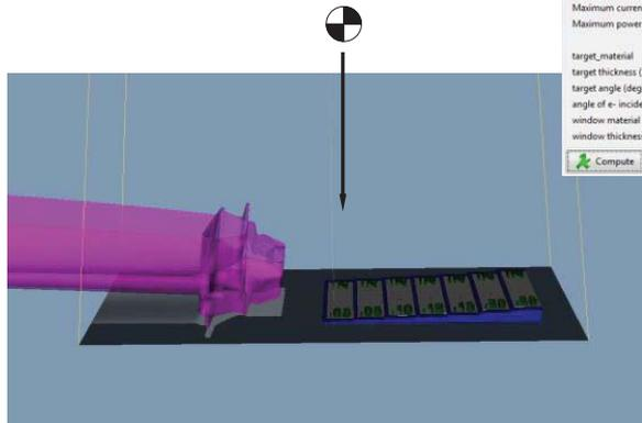
Simulation of the X-ray image with the same parameters for tube, film, and geometry as in reality.
