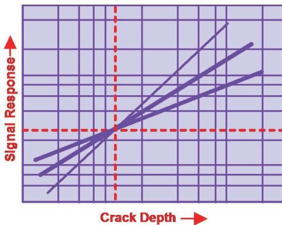
Figure 7. Signal Response Variances Using A Single Point “Calibration”
