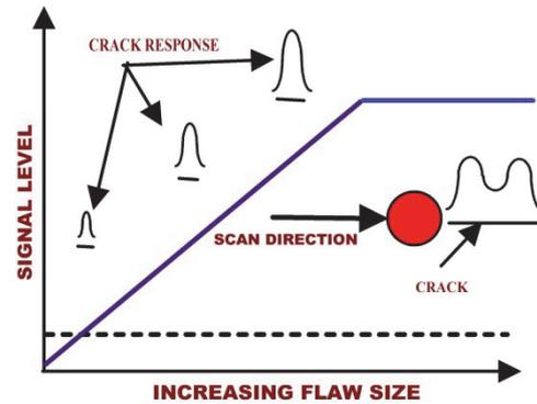
**Figure 10.** Eddy Current / Crack Interaction
