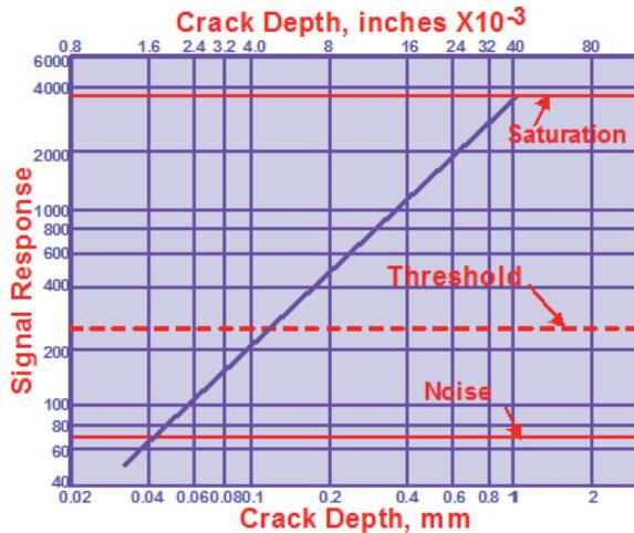
Figure 9. Data Form for the Berens Model
