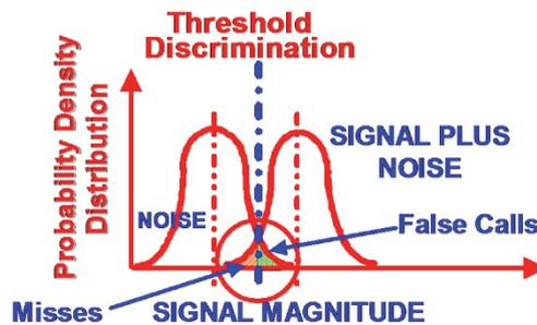
Figure 6. Overlapping Signal and Noise
