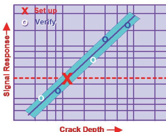
**Figure 8.** A Multiple Point ‘Calibration’ and Response Verification
