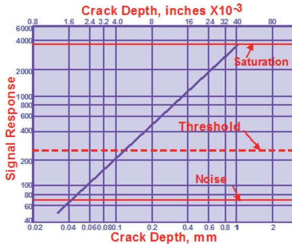
**Figure 9.** Data Form for the Berens Model
