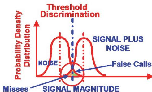
**Figure 6.** Overlapping Signal and Noise
