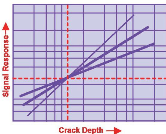
**Figure 7.** Signal Response Variances Using A Single Point ‘Calibration’
