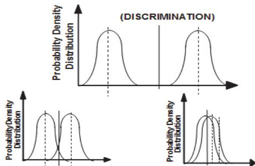
**Figure 5.** Reduced Discrimination at Smaller Flaw Sizes
