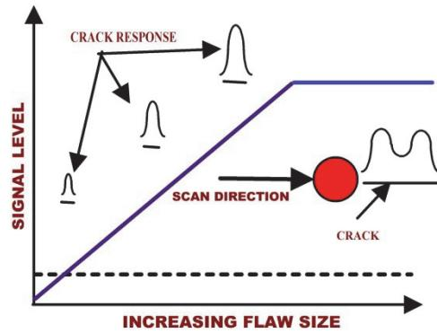
Figure 10. Eddy Current / Crack Interaction
