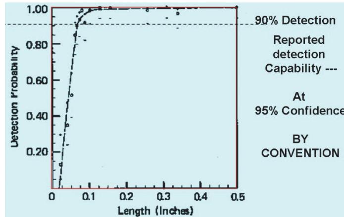
Figure 3. A POD Curve from the Original NASA Program
