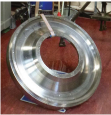
An aerospace engine titanium disk to be loaded into the immersion tank. The component is approximately 1m in diameter. Note the different surfaces of this intermediate form, which are all individually scanned, often at more than one probe angle.
