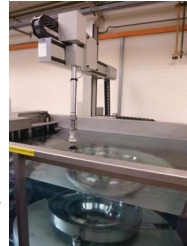
The disk in the tank, positioned on a turntable below a manipulator arm used to position the ultrasonic probe. To permit access to the under surfaces of the disk, the component is flipped half-way through the inspection.
