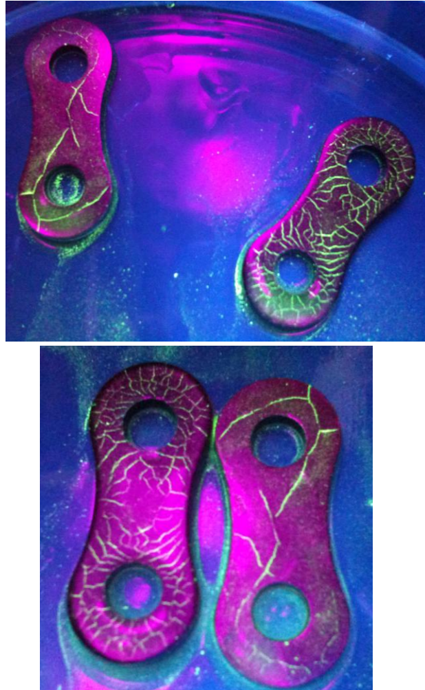
Fig. 1. Defects found out on the surface of a plates with suspension application, prepared on the basis of a concentrate of fluorescent magnetic powder “Diagma -1613”.
