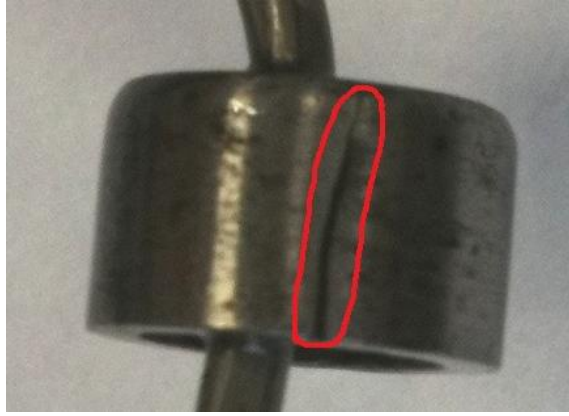
Fig. 2. Defects found out on the surface of a roller with suspension application, prepared on the basis of the black magnetic powder.
