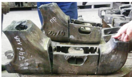
Pic. 1. Cutting of side frame №742; in zones, marked by results of testing by method M2 internal flaws were not detected
